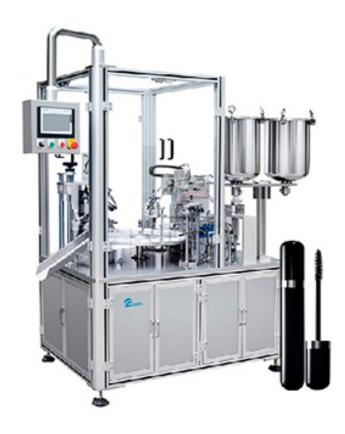
JRM is a kind of automatic filling machine for mascara and lip gloss. The process section is including auto filling, steel ball inserting, blush inserting and capping device.
