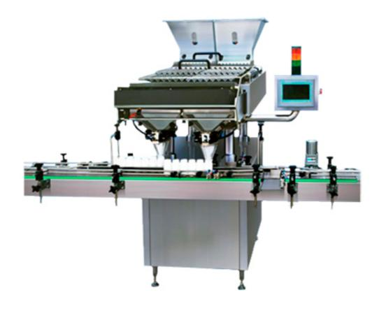
It adopts the channel vibration to feed in uniform speed, working reliable, stable and lower noise. BPS-D16 uses three-stage vibration plates.
