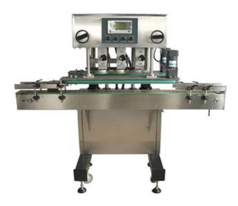
GX200 is economical, and easy to operate. This versatile in-line capper handles a wide range of containers at speeds up to 200 bpm and offers a quick and easy changeover that maximizes production flexibility. The tightening discs are gentle which will not damage caps but with a excellent capping performance.
