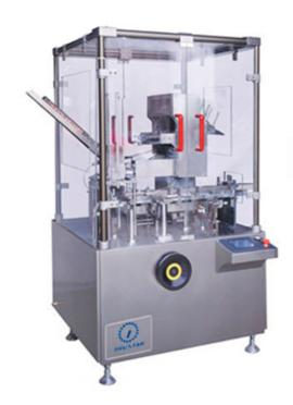
This machine is suitable for feeding and encasing of the blister plate. It consists of leaflet folding (1-4 folds) and feeding device, carton forming and feeding, batch number printing, sealing of case tongues at both ends etc. The whole encasing process is finished automatically. A hot-glue machine can be added to it.
