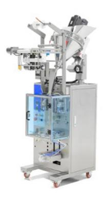
CBZ-50F automatic single-row powder back-seal packaging machine is a small vertical packaging machine designed for powder products. The equipment adopts advanced computer control technology and can realize fully automated bag making, metering, filling, sealing, printing production date, tearing, cutting and counting processes. It is suitable for the packaging needs of powder products in the food, chemical, pharmaceutical and other industries.
