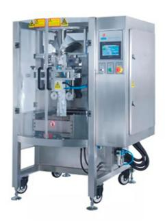
The HSC-560 packaging machine is a continuous motion vertical form fill seal packaging machine. It incorporates a unique sealing motion based on a hypocycloidal geometric path, to provide extended seal dwell time with a smooth, natural trajectory motion. Speed up to 180 bags per minute.
