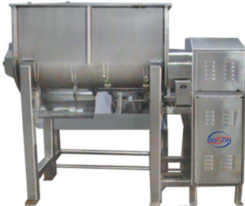
Our Ribbon Blender are designed in such a manner so that even the smallest quantity of ingredient can be blended efficiently with large volumes. Being a client centric organization, we manufacture and supply a premium quality range of Ribbon Blender that are used for blending of various materials in a fast and efficient manner. The Ribbon Blender is an efficient and versatile blending machine for mixing and lubrication process of dry granules and powder homogeneously.
