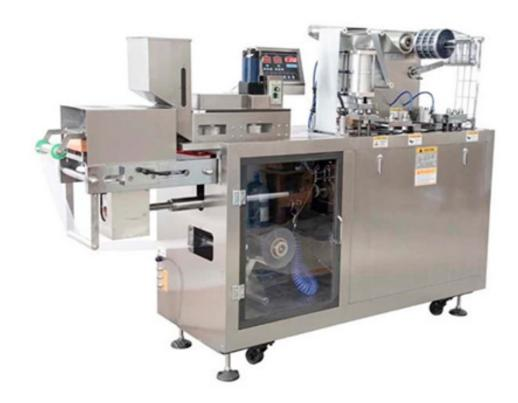
The DPP-150 flat blister packing machine is suitable for sealing capsules, tablets, sugar coated, capsules, injections, shaped products, as well as medical devices, light food products, and electronic components with blisters.
