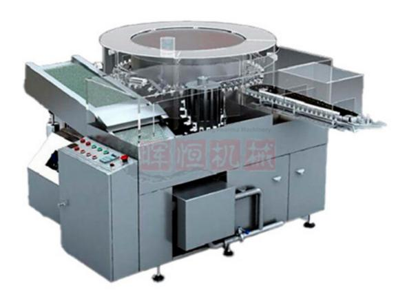
SHH-QCL series automatic washing machine consist of infeeding section, ultrasonic treatment section and final washing section, the containers are going through those sections for completion of the whole washing processing by Ultrasonic treatment, prewashing and final washing steps, the cleaning quality of the container washed meets any Pharmacopoeia and being able to validate.
