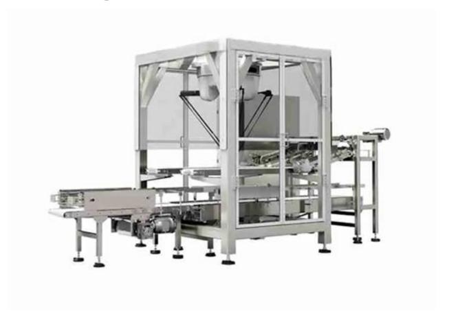
This machine introduces advanced parallel robot (spider arm) and corresponding software control technology. It is used for automatic gripping and packaging of soft bag products to open empty cartons. This machine is mainly applicable to the packaging process of milk, water, beverage, oil and powder production lines, as well as the packaging of various shapes of products in other industries.
