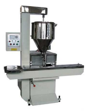
There is one hopper of 35 kg with heater mixer on the machine, and there is also one heater on the pipe and filling nozzle, so the machine is applied to fill various viscous materials, such as lipstick, Adhesive, crayon, foundation cream and ointments and so on.
