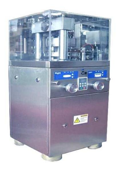
ZP-5 is a new generation product by our factory, and this machine is a single Roller continuous automatic tablet press for pressing various kinds of different shape tablets and plain tablets. It is mainly used in pharmaceutical industry and also the chemical, food, electronic industries.
