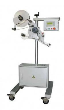
Labeling machines are applied to various operations such as sticking a label on plane, post surface, single side or multi-sides of a package, sticking labels covering part or all of the surface of a cylinder, or sticking on sunken locations and at edges or corners.
