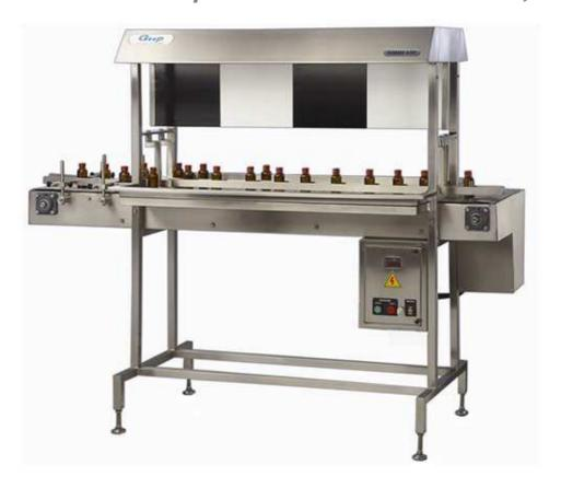
Inspection table is equipment consisting of a three-track conveyor with a hood with lighting arrangement and visual inspection background of alternate black & white color. Inspection table have stainless steel structure with moving S.S. slat chain. Structure made out of S. S. square pipe & supported on adjustable bolts.
