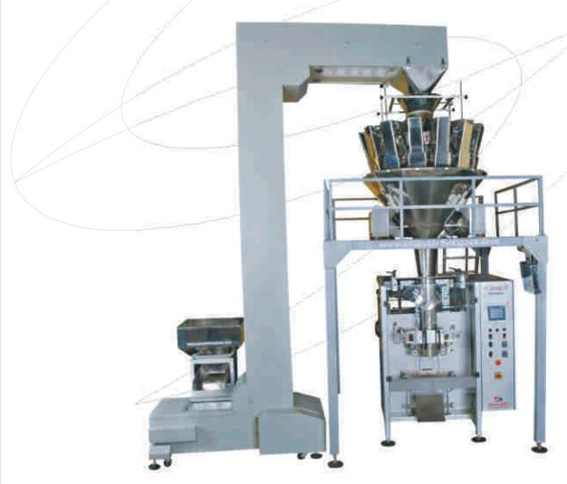
Kawach Servo Machines are very high speed machines of international standards with all precision. The high end CPU motion control technology gives the highest speed up to 100 pouches/min. (Depend on product material characteristics & pouch size). All operations are handled by individual servo motor. Kawach servo machines are designed only for large scale manufacturer. These machines run at high speed with high weight accuracy & sealing intactness.
