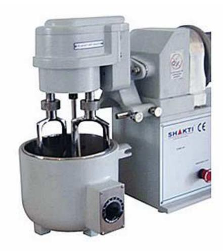
Double Planetary Mixer SDPM is designed to mix products including adhesives, ointments & creams pharmaceuticals, foods, chemicals, electronics, plastics and pigments. This mixer is provided double mixing paddle. This mixer is ideal for mixing and kneading viscous pastes under atmospheric or vacuum conditions. Capacities 3 to 3.5 kg. Many options including jacketing for heating or cooling, vacuum or pressure etc. are available. The kettle is also easily removable.
