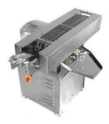
De-foiler is one of the small but needful machines. It is ideal for recovering the tablets, Hard Shell capsule from the rejected & unsealed strips without any damage and such recovered Tablets/Capsules can be replaced on strip packing machine.
