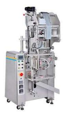
3-side sealing. Dosing by material volume; applicably for small quantity packaging, pellet or powder material. Such as powder soup / spice, cereal powder, juice powder sugar... etc.
