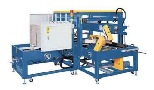
The CHS-6801 is a Vertical type Automatic Carton Erector. These systems fits for automatic production line. It erects cases of different and sizes and it seals the bottom side of carton with tape or hot glue on demand.
