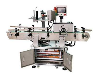
Applicable to variety of regular rpunnd bottle or a small taper round bottle, paste one or two labels, which can be widely used in attaching to the full circle and semi circle labeling
