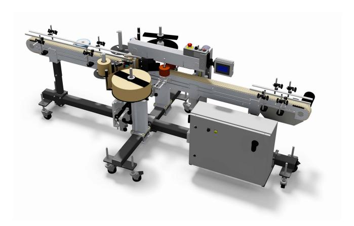
ID Technology's LSI-9150 is an in-line labeling system for applying one or two labels to non-round containers at a rate of up to 120 per minute. The addition of an optional wrap-belt, allows labels to also be wrapped around round containers.
