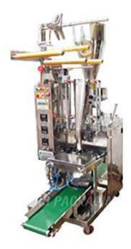
The MK-201 is a semi pneumatic vertical form fill and seal packaging (VFFS) machine designed to package granular and free flowing powdered products. This machine uses volumetric cup dosing system to produce center sealed and 3 side sealed pouches / bags.
