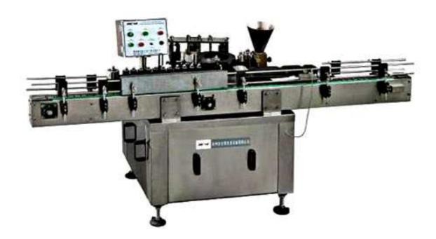
It is applied for the long or circle labeling, delivering labels, delivering bottles, pasting and labeling are finished at a time automatically. Operation easily, the place of labeling is uniform and orderly. It can use the common paper label and debases the producing cost.
