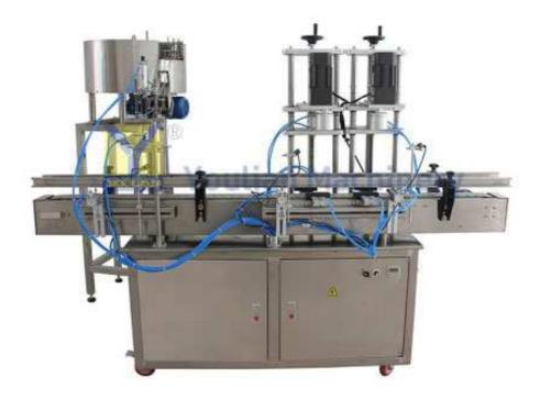
This is a automatic capping machine. The bottle is conveyed in a straight line and then capping. For high-volume products, it is suitable for round caps of various sizes and shapes. Widely used in food, beverage, daily chemical, pharmaceutical and other industries.
