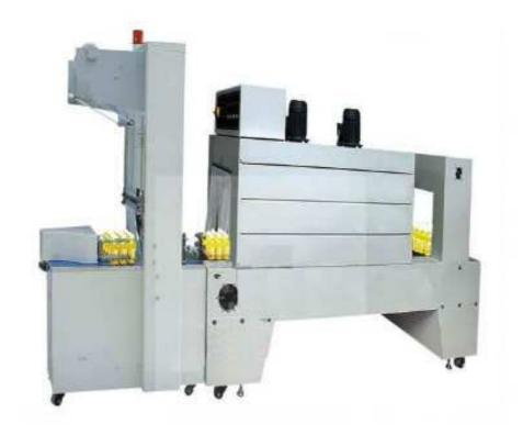
BZJ5038 series sleeve wrapper is suitable for wrapping pop-cans, bottles, etc, both with bottom-tray and without bottom-tray, working with BSE-5040A or other PE shrink tunnels.
