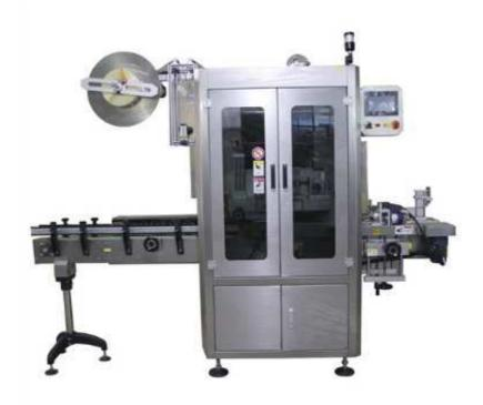
Automatic plastic bottle shrink sleeve labeling machine adopts PLC programmable controller, imported servo motor, servo driver, frequency converter and transducer; besides, this bottle label machine adopts the positioning module to ensure the casting label precise, rapid and stable. Our bottle labeling machine not only has a highly precise position for casting label, but also can withstand the perfect shape of the bottle after shrinkage.
