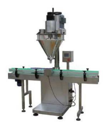
All the work of measuring, filling can be done automatically. The machines have special design, so that especially suit for filling the power which is easy flow or poor liquidity. Such as: veterinary drug, sugar, solid chemical, spice, talcum powder.
