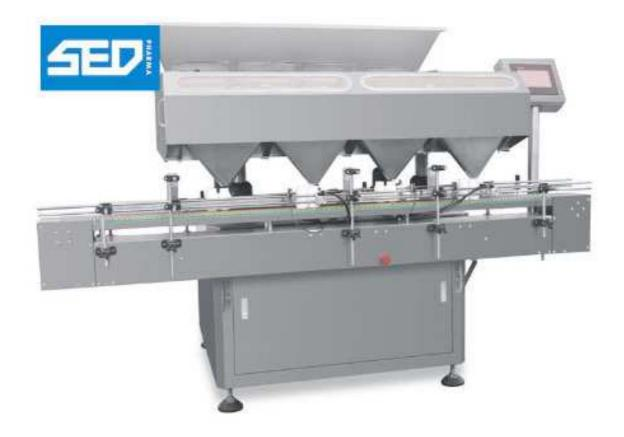
SED-32S Automatic Electronic counting machine is special for counting tablets, soft gelatin, hard capsule and chewing gums, etc. This machine adopts 32 sets imported counting sensor for counting with 32 Guiding Way and two head. The advantage of the machine is no need change mould when you change the counting object, only adjusting the counting table height by Easy Adjust wheel. The machine comes with Touch screen operation and PLC Control for convenient running.
