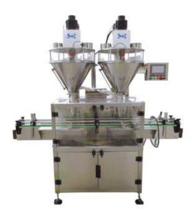
This machine is mainly controlled by mechanical, electrical control, conveyor belt, photoelectric detection, powder filling device, a bottle body, a touch screen. The powder or granule feeder can choose by yourself.
