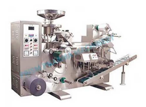
Automatic Blister Packing Machines are ideal tools for the pharmaceutical industry for the packing of Oral tablets, capsules, hard and soft gelatin and ampoules. All machines are manufactured under stringent quality control process to ensure years of trouble free production. Special design of machine ensures total synchronization of timings between sealing of Aluminum foil and PVC base web. The machine works on the flat forming & rotary sealing principle for delivering higher outputs.
