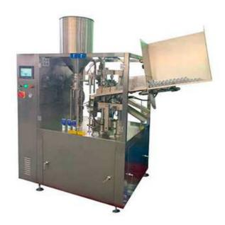
Automatic plastic tube filling and sealing machine is widely used in pharmaceutical, food, daily cosmetic and chemical industries. It can seal both plastic tube and plastic aluminum laminate tube.
