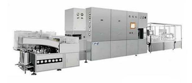
This vial filling line contains processing of feeding, washing, drying, filling, plugging, capping. The line meets GMP requirement with high efficiency and anti-leaking function. Easy operation with PLC controlled and adjustable parameters in touch screen. Each machine can be used standalone, also can be used for filling line.
