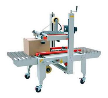
The FXJ-6050 is complementary to the FXJ-5050. The top and bottom driven mode of the machine can pack larger and heavier goods, and there is no limit to the maximum length of the carton.
