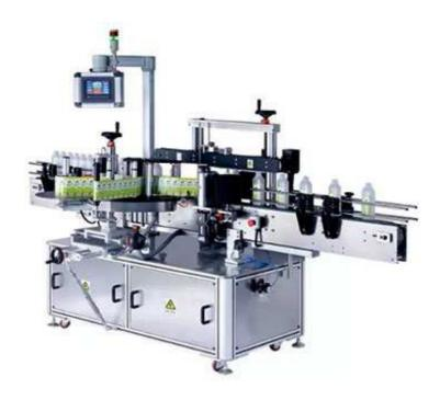
The one-sided automatic labeling machine is suitable for side labeling of square or flat bottle shaped objects.
