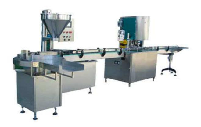
This powder filling and sealing machine is specially designed for automatic filling and capping bottles with powders and small particle substances. It can do various work like automatic positioning, filling and measure capping of the bottles.
