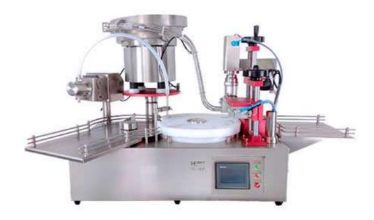
XQXG-30S is a ready-to-use fully automatic filling and capping system, suitable for biotechnology Clinical trials and small batch sample production in the fields of technology, pharmaceuticals and diagnostic reagents.
