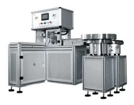
This blood tube capping machine is used for EDTAK2, EDTAK3, Heparin tube capping.
