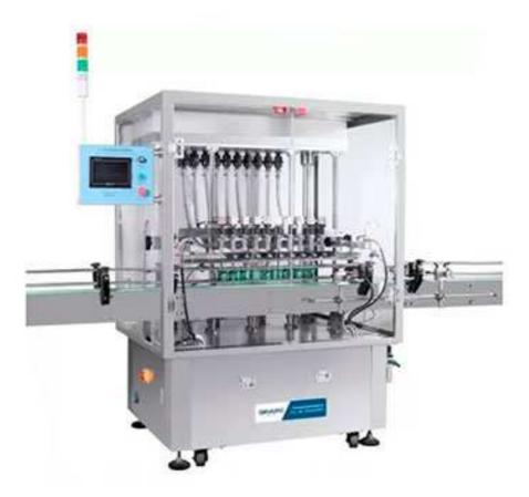
The fully automatic filling is servo motor detergent filling line that is designed to fill bottles and jars with products of various viscosity, ranging from water thin liquids to thick creams. They are used in the cosmetic, food, pharmaceutical, oil and specialty industries. These inline piston filling machines come complete with: two to twelve fill heads, a variable speed drive conveyor, adjustable heavy duty stainless steel frame, an easy to operate control panel.
