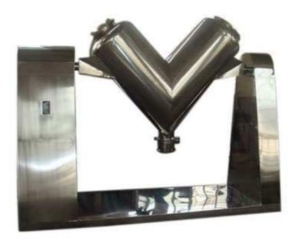
This machine is suitable for mixing two or more dry and powder or granule raw materials from pharmaceutical industry, chemical industry foodstuff industry and so on.
