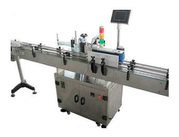
Automatic labeling machine for the application of labels on round bottle. The machine is composed by a conveyor, one of label adaptor and one of label applicator. In case of wrap around label application a side conveyor is installed. There is also the possibility to install a hot stamping unit, print expiry date, batch code etc. The bottle loading/unloading can be done manually, through loading/unloading turntable (alternative Ø620mm or Ø900mm) or directly from an production line.
