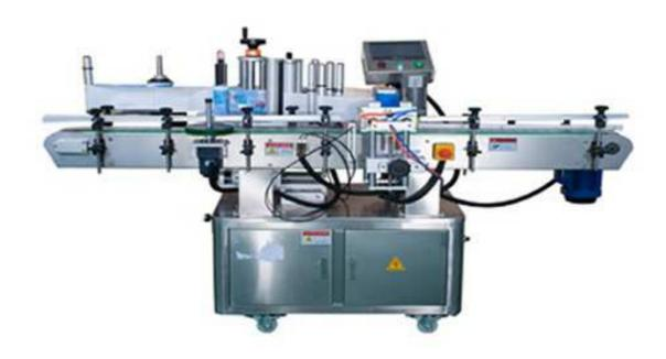
Applies to the circumferential surface of the object class round bottle labeling, can be attached to a single standard and double standard, are back double standard spacing can be flexibly adjusted, such as gel water round bottles, cans and other round food labeling, widely used in cosmetics, food, pharmaceuticals, disinfectant and other industries.
