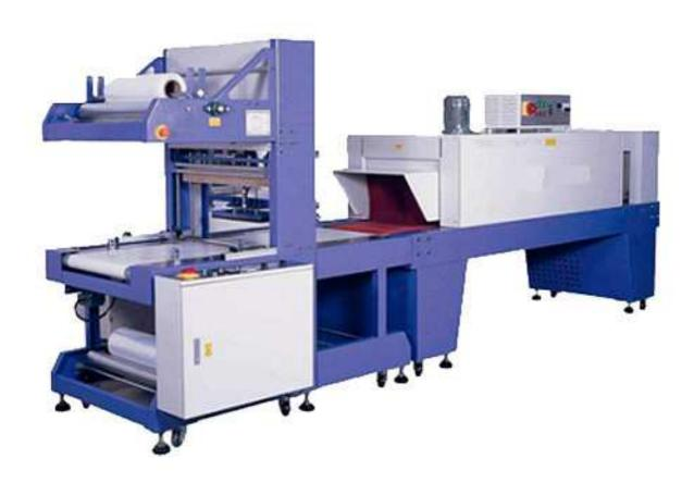
The automatic sleeve wrapping machine is suitable for wrapping and then shrinking cylindrical products like bottles, cans, boxes, big cartoon, bags, etc with or without bottom tray. The whole process of sealing is mainly conducted in two steps
