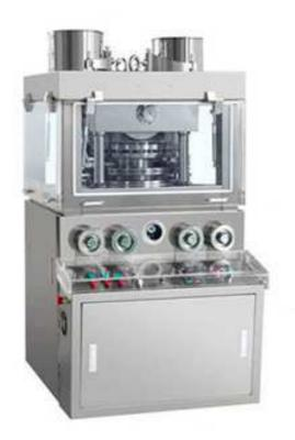
This machine integrates automatic rotation, frequency-conversion, speed-adjusting with continuous tablet-pressing.
