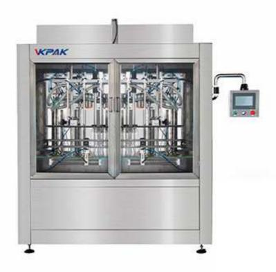
Hand sanitizer is moderately thicker than water making it ideally suited for piston fillers. The VKPAK series fillers can fill up to twelve containers at a time. Switching from filling two, eight or sixteen ounce containers can be done in minutes without tools.
