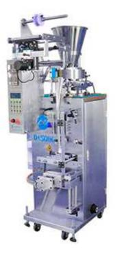
Double transducer control, flexible bag length cutting, operator needn't to adjust the unloading working, saving time and saving films.
