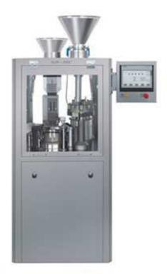
NJP-400C Automatic Capsule Filling Machine adopts butterfly valve-type powder feeding, and is very suitable for drug powder with poor liquidity, including Chinese herbal medicine and Chinese patent drug, due to that its vibration unit equipped will force the powder to run down, which has solved problem of failing to feed in powder that often happens in the traditional screw feeding device because of the poor liquidity of powder.
