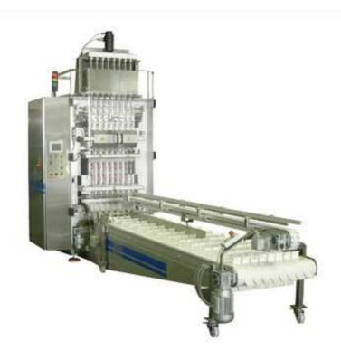
It is a full automatic machine to make package and filling of the products to these packages. Lots of applications that can provide product flow are possible. Sensitive filling can be done due to the fact that product filling is controlled by servomotors. Especially, with the applications in food sector, its high capacity, and product output quality, it provides advantages to the users.
