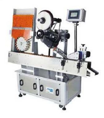
The Horizontal Labeling Machine is suitable for the labeling of various round bottles that cannot stand up. It can be equipped with, feeding and labeling structures according to customer needs. The body can be designed to tilt forward or backward. It is suitable for small round bottles. The diameter can be determined by the product.
