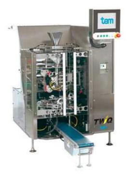
This Vertical Form Fill Seal Machine (VFFS) machine can be used to handle flat-bag, quattropack, and three-sided seal bag. It has robustness following the vertical pillow-pouch filling machine, and moreover, is capable of handling diverse product shapes and still fit within confined space. Changeover from flat-bag to quattro pack is easily possible by swiveling the end-seal unit.
