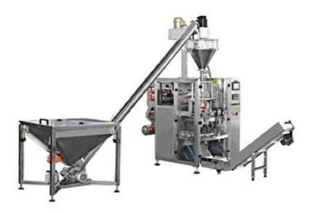
The screw metering method is used for bag packaging of powder materials and powder materials with a particle size larger than 200 mesh. All materials in contact with the material are made of stainless steel and non-toxic, wear-resistant plastics that meet the requirements of food and pharmaceutical packaging.
